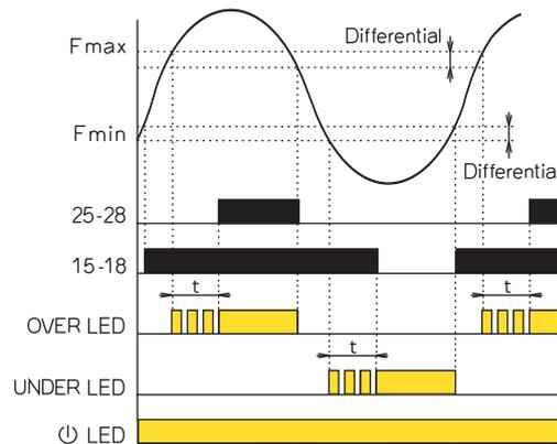
After the supply (monitored) voltage is connected the green LED is on.
